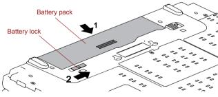
Figure 6-2 Securing the battery pack
